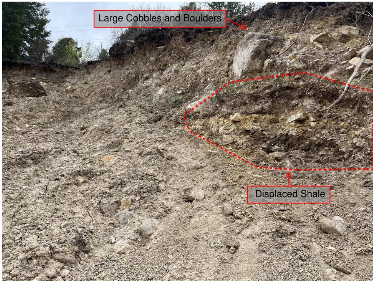
Figure 7 – A close up view of the slide materials in the right (northwest) flank of the recent 2025 slide scarp. Blocks of maroon and ochre displaced shale are circled on the right. This shale could have been incorporated into glacial materials by translational sliding. Also shown is the amount of variation within the size of material within the scarp, ranging from very fine clays and silts up to large boulders and cobbles.
