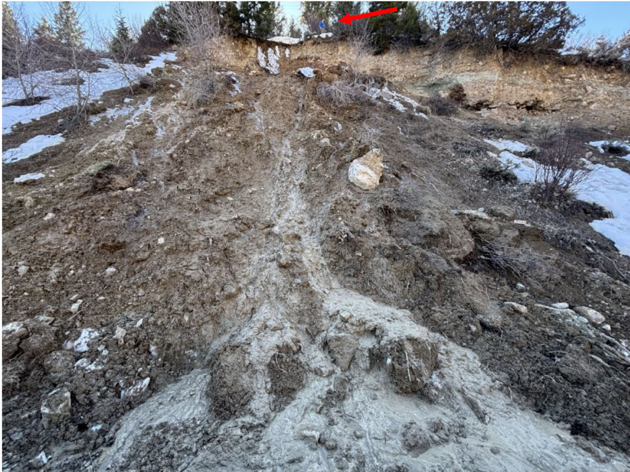
Figure 6 – A west facing view of the landslide taken from the toe. There is a person in a blue jacket at the top of the slide, marked by an arrow. The head scarp is approximately 10-20 feet tall. Some cobbles and boulders are seen coming down the slope. The slide debris in the foreground has a soft and saturated consistency due to the amount of water exiting the slide face.
